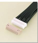
This is a 2.0 mm pitch dual-row wire-to-board connector. With a mounting height of 8.8 mm and a depth of 5 mm, the low-profile, space-saving design supports the miniaturization and high-density design of devices.
