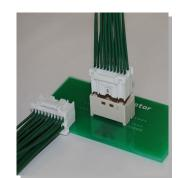
This PID connector is a 2.0mm pitch box type wire-to-board connector with secure lock device, and it has the mechanism for detecting half mating, which is possible to judge electrically whether its state is the complete or incomplete mating by the circuit of detecting half mating provided at the center part of connector.
