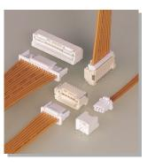
This is a 1.5 mm pitch wire-to-board connector with a solid locking feature for high-density board design. Ease of mating is facilitated with a low insertion force and a positive tactile clicking sensation, providing a highly reliable connection.
