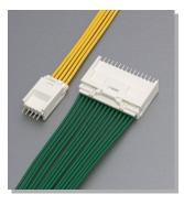
This is a board-to-wire connector with secure locking device that has been designed to 2 mm pitch high box type, with a mounting height of 19.95 mm (including retainer) and 6.65 mm in depth. Low insertion force type contact is adopted and it provides excellent operability. Retainer is available as usage.
