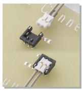
This connector is compact and low profile type, height 1.2mm and width 4.7mm, 1.2mm pitch wire-to-board connector.
