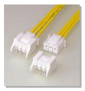
VU connector is small type 3.96mm pitch PC board connector for large current and has the high reliability in a power supply circuit, considering the fully shrouded connector header structure against "vibrating connector" and "distored extraction".
