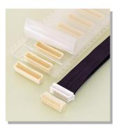
\*Compact, double-row design \*Although this shrouded header has locking features for its mating receptacle, there are no holes in the header shroud that would adversely effect vacuum gripping equipment. \*The receptacle has protrusions on both ends for an operator to disengage the receptacle from the header without holding the wires the wires.
