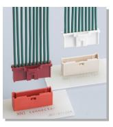
This connector is 2.5 mm pitch wire-to-board connector that has a mechanism to prevent an incomplete mating by utilizing the inertial force when mating connector. In all circuits of connector, controlled key for preventing mismatching of mating is added, and two type connectors can be used in the same model.
