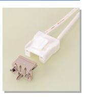
Can be connected to vinyl insulated flat cables (such as SPT, HVFF) ranging from AWG #20 to 16 which are used for primary sides of power circuits. \*PC board locking device makes temporary mounting and correct positioning onto the board easy. \*Misinsertion preventive construction and arm-lock mechanism.
