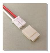
This is wire-to-board connector for LCD backlight power supply. The board occupied area is smaller than our BHS connector designed for the same purpose, and the mounting height is 13% lower than the BHS, achieving 2.8 mm.
