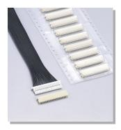
This is an ultra-thin 1.0 mm pitch wire-to-board connector for thinner and smaller devices, with a mounting height of 1.8 mm for the normal type and 1.4 mm for the offset type.
