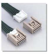
This is XM connector high box type, with 20.0 mm mounting height and with 8.9 mm thickness. This connector exhibits the stable electric connection to the condition such as the vibration, the prying, the micro-current and micro-voltage circuit.
