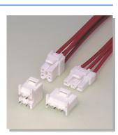
This VYH connector is designed for wire-to-board 6.5 mm pitch connector corresponding to large current. Retainer, which prevents from insufficient insertion of contact and coming off contact, may use and large current circuit can be connected certainly and safely.
