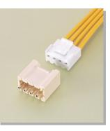
The header is tall and fully shrouded so as to prevent the resin used to coat the PC board coming into contact with the mating pins. Designed for use specifically with resin coated ("potted") PC boards. \*The header is designed to accept VH mating receptacles. \*The heaving has a lock mechanism which prevents the
