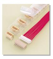
This is a 1.5 mm pitch wire-to-board connector with 5.9 mm in mounting height and 3.5 mm in depth when mated with the top-entry type through-hole header. The housing lance design improves contact insertion workability. In addition, the combination of high contact force and round pins provides stable contact performance.
