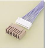
This is a XH connector high-box type with a mounting height of 17.0 mm and a thickness of 5.8 mm. It provides stable state contact even for micro-voltage and current circuits.
